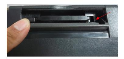
2. Connect the self-testing plug into the tech2 module.
