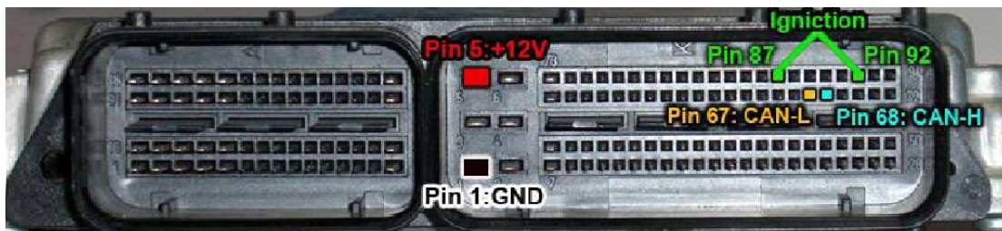
Picture 1 MED17.1 terminal
