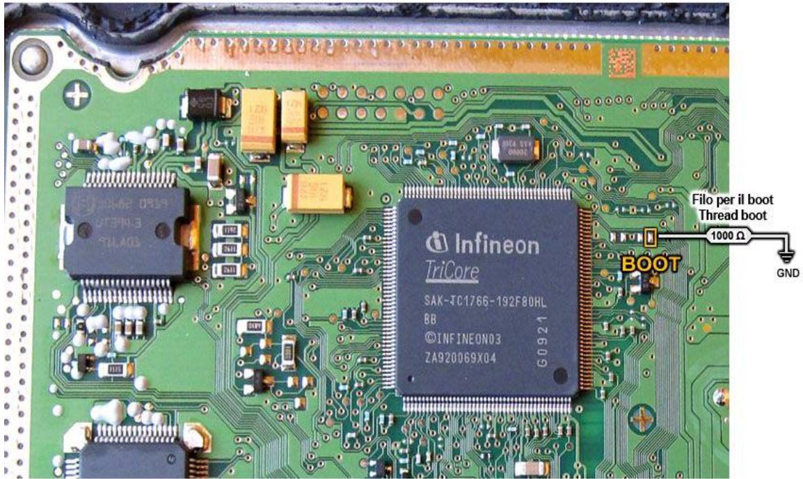
Picture12 MED17.5.5 PCB
