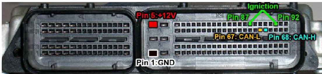
Picture11 MED17.5.5 terminal
