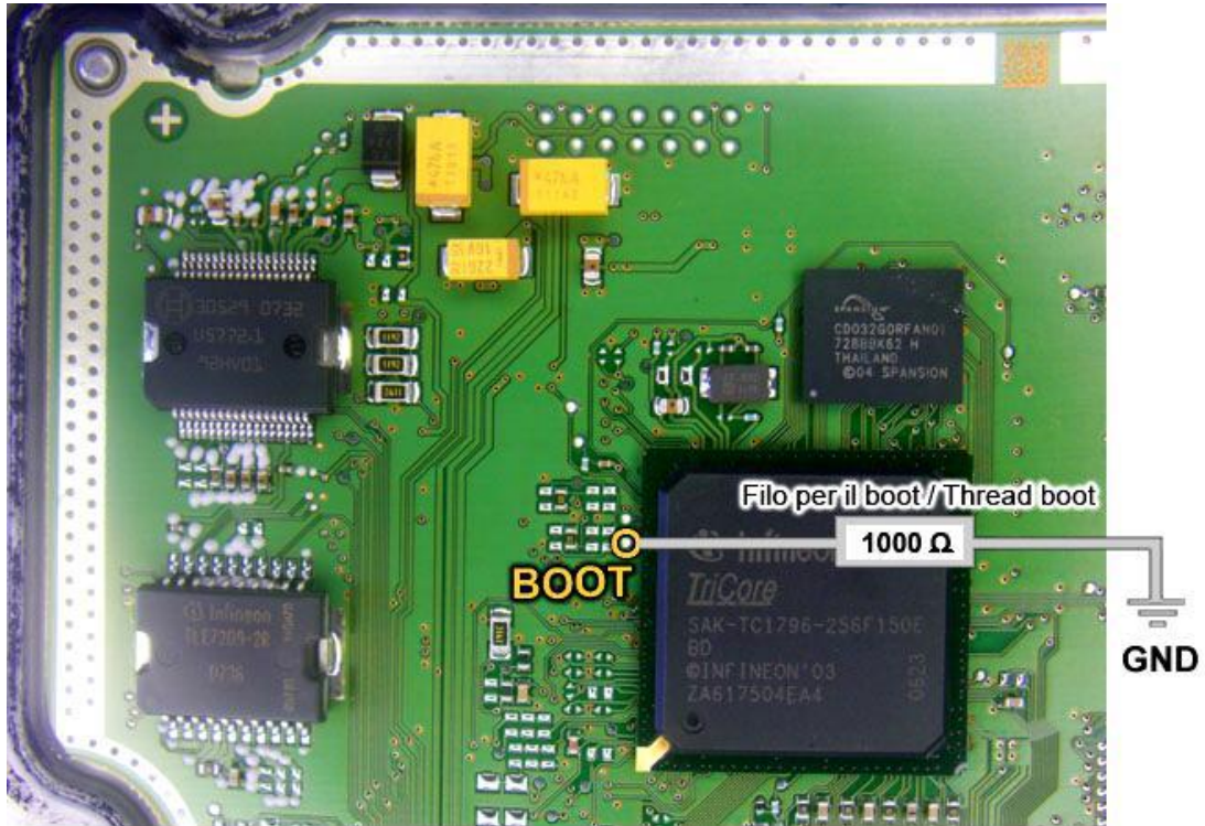
Picture8 MED17.5.1 PCB
