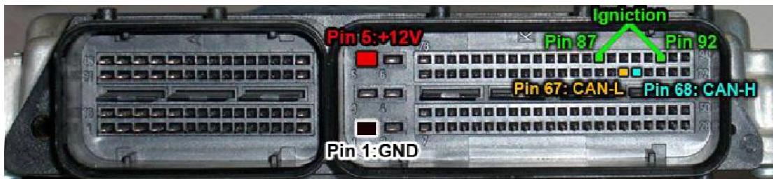
Picture9 MED17.5.2 terminal
